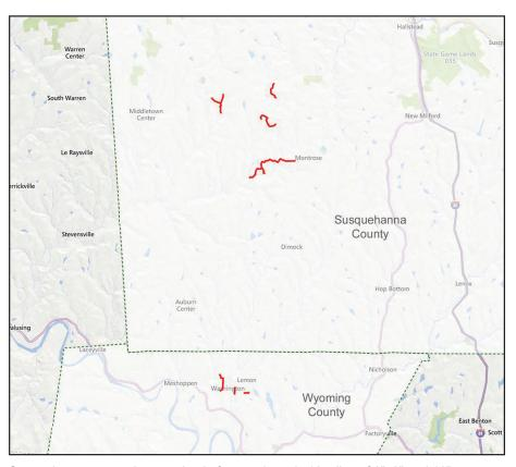
Susquehanna county is comprised of approximately 12 miles of 6", 8" and 10" natural gas gathering pipelines operating at 500#. Wyoming county is comprised of approximately 3 miles of 8" and 10" natural gas gathering pipelines operating at 1200#.
